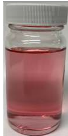
Photo 2 - Colour after mixing 20% AVGAS 100 LL blue + 80% WA 91UL red
